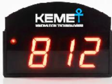
**14****KQS207****3 Digits Wired – Ethernet RJ45 Connection – POE 12 V DC**
